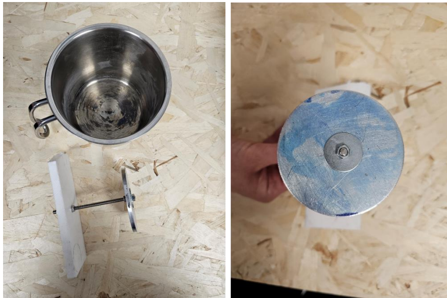
Figure 12: Container and electrode used for the measurement.
