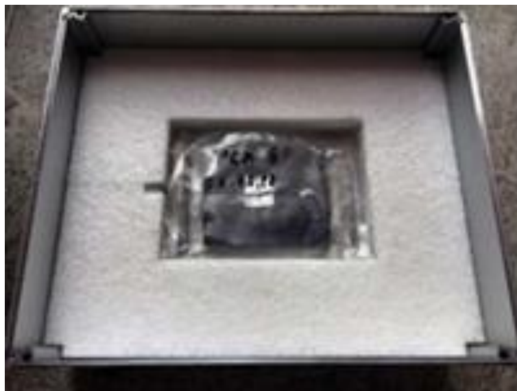
Figure 3: sample insertion in calorimetric measurement device [2]
