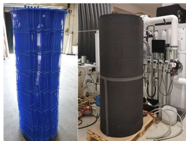
Figure 5: 600 l storage tank with capillary plastic HEX (left),
