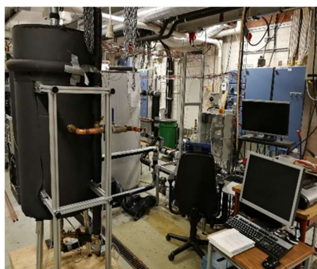
Figure 6: The prototype of PCM heating solution developed at KTH.
